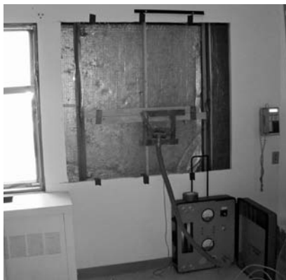
A Air leakage testing can identify components in need of increased airtightness to improve energy efficiency.
