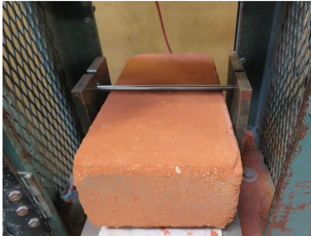
Figure 9. A splitting tensile test set up on an A3 series block prior to loading.
