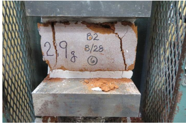
Figure 16. A B2 series block after loading to failure during C67 testing.
