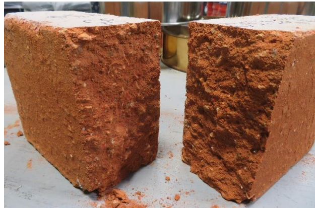
Figure 12. A B2 series block after a splitting tensile test.
