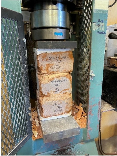
Figure 17. A2 series prism 6-5-6 prior to C1314 testing.
