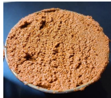
Figure 33. Dry side of optimum moisture density.
