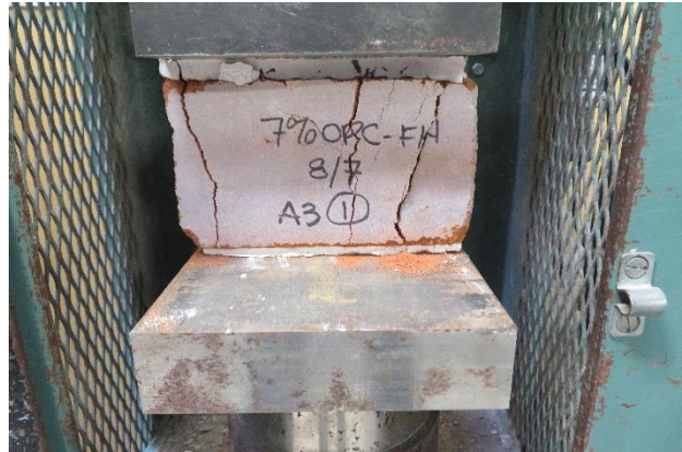
Figure 14. An A3 series block after loading to failure during C67 testing.
