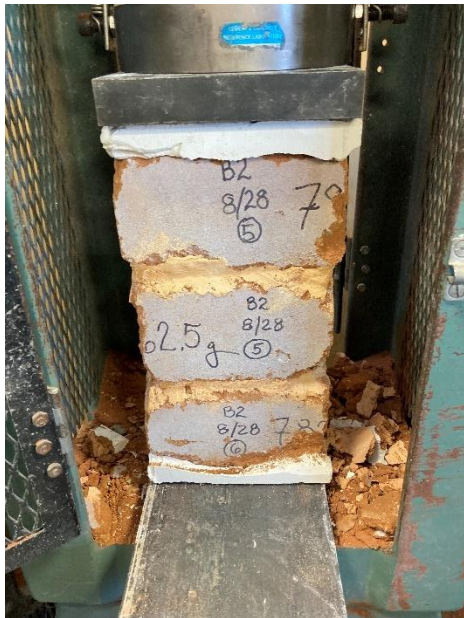
Figure 19. B2 series prism 5-5-6 prior to C1314 testing.
