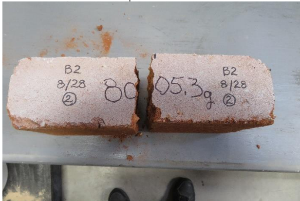
Figure 11. Side view of a B2 series block after a splitting tensile test.
