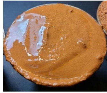
Figure 31. Wet side of optimum moisture density.
