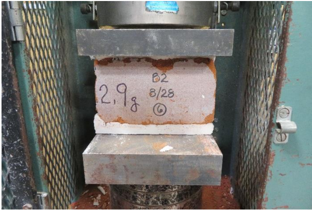
Figure 15. A B2 series block during C67 testing.
