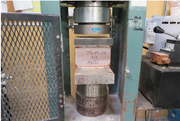
Figure 13. An A3 series block during C67 testing.
