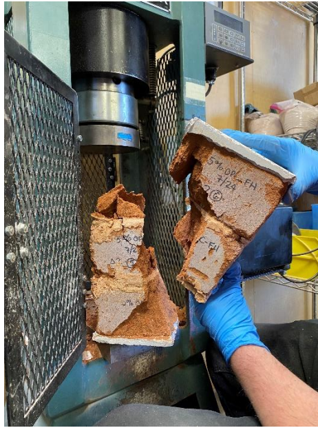
Figure 18. A2 series prism 6-5-6 after C1314 testing, and being dissected to determine the failure mode. The failure mode was classified as "cone and shear".
