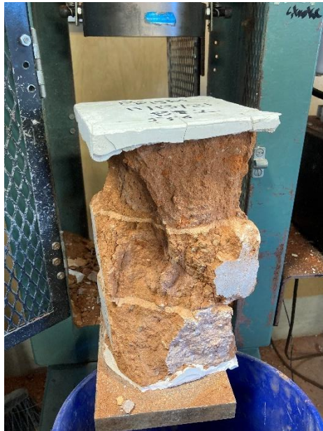
Figure 20. B2 series prism 5-5-6 after C1314 testing, and being dissected to determine the failure mode. The failure mode was classified as "cone and split".
