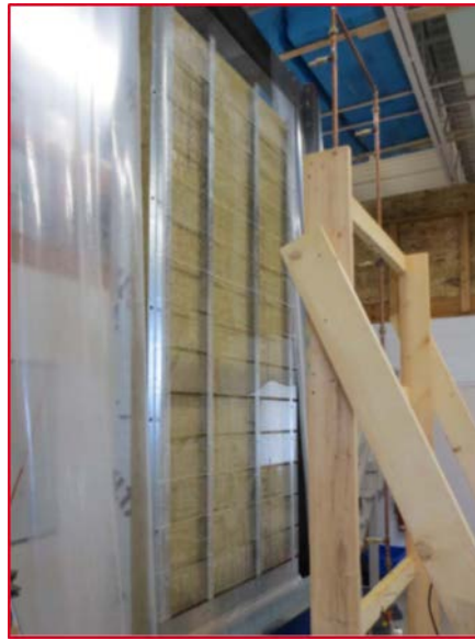
Stonewool test wall assembly behind open joint plexiglass cladding
