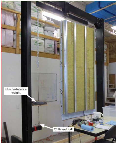
Stonewool test wall assembly hanging on drainage balance apparatus
