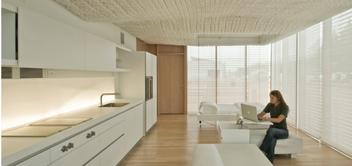
Figure 10: Interior of main living space with internal and external shades deployed and light diffusing soffit above. Ambient canvas delivers haptic information at kitchen backsplash.
