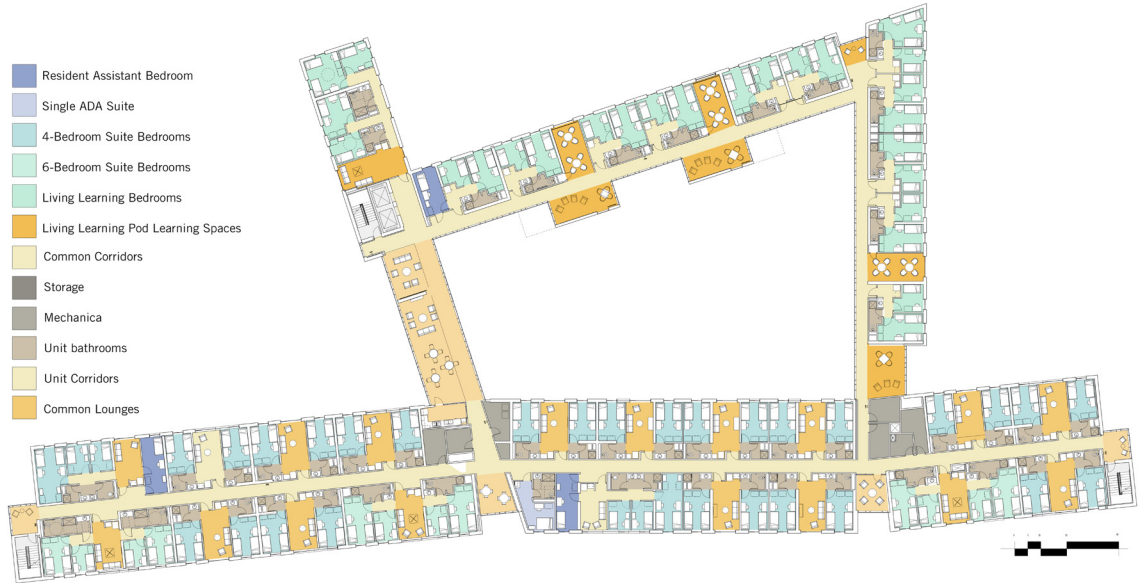
Figure 2: Typical Residential Floor plan—Located on East Campus, the hub of residential life on campus, the 500 beds are grouped in two prime categories: suites and living / learning pods. The suites are programmed in three types that include 4-bed doubles, 4-bed mixed singles and doubles, and 6-bed mixed singles and doubles. Twelve Residential Assistants' suites are split among the three residential levels. A Residential Director apartment at ground level has private access, which is also connected to the rest of the building.
