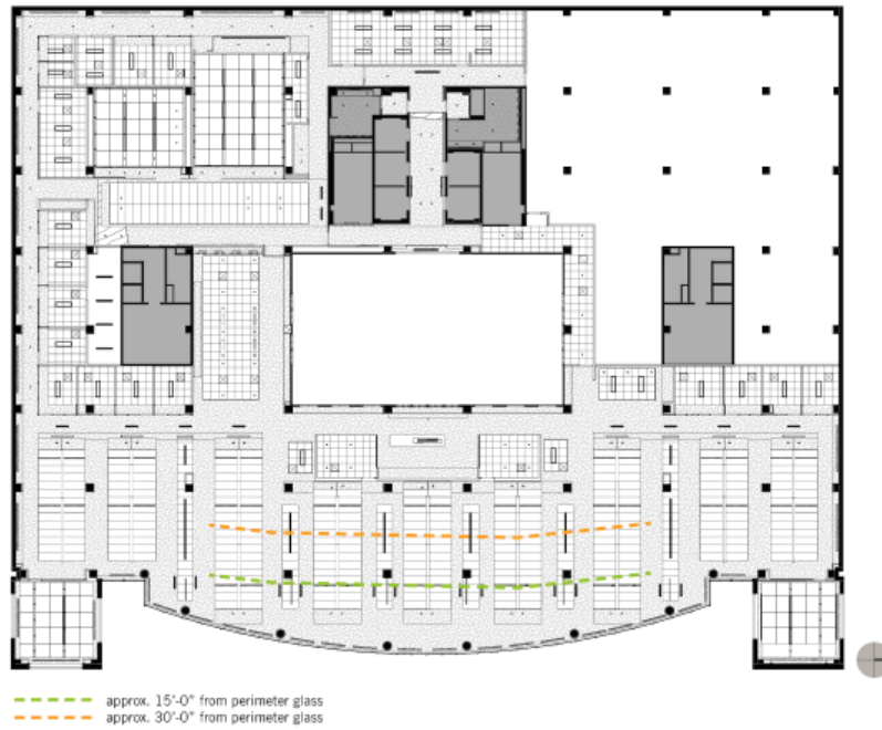
Figure 13: Diagram for recommended daylight harvesting locations.
