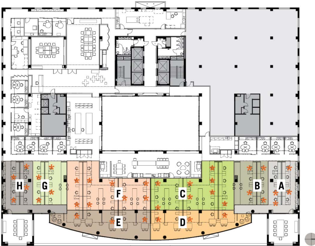
Figure 2: Zoning diagram for lighting level data collection.
