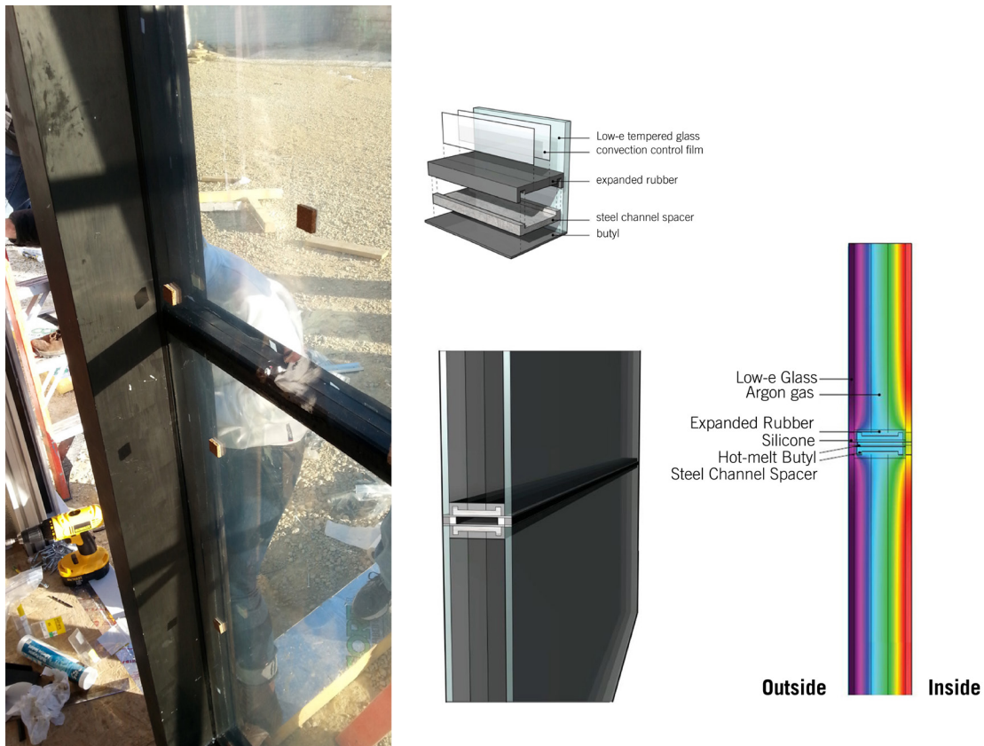
Figure 5: System A prototypes and thermal simulation.
