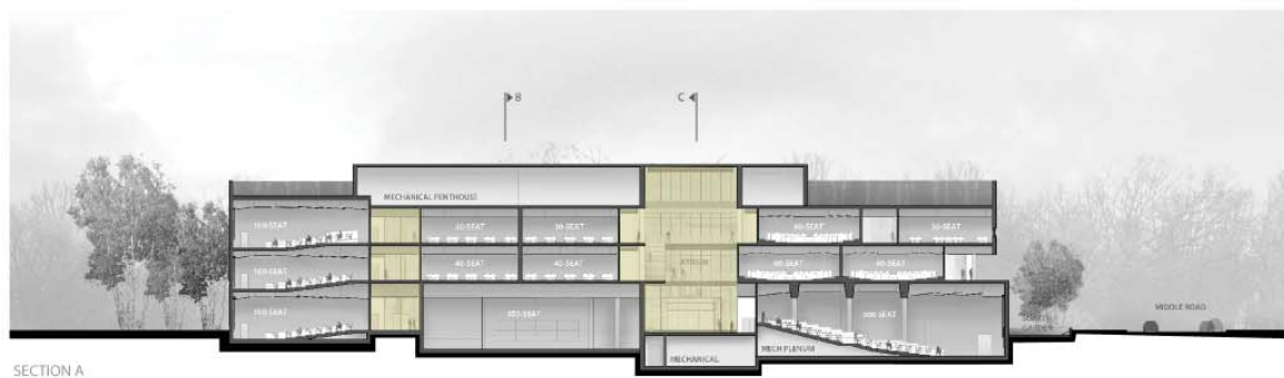
Figure 8: IC UTM spatial configuration (internal, interstitial and peripheral spaces).
