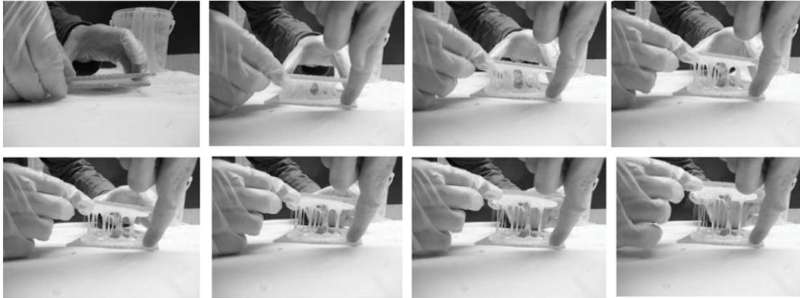
Figure 1: Using plates and pulling as a technique to create the material structure<sup>4</sup>.
