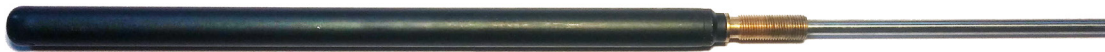
Figure 3: A thermal actuator, used in this study. The body on the left contains wax or oil that expands when exposed to heat. The piston on the right creates a “stroke”, pushing out due to this expansion.
