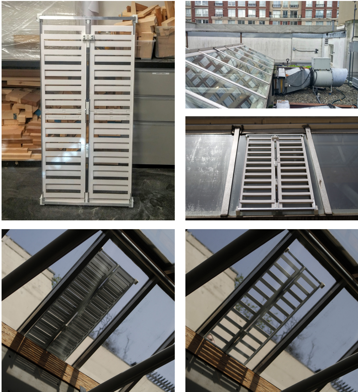
Figure 12: The completed prototype placed in position on the test site. Bottom Left: Temperature above 20°C (59°F). The ambient air temperature closes the shutter and limits solar gain. Unfortunately, Vancouver has not had a sunny day in over two weeks at this point. Bottom right: Apparatus installed, visible from below. Temperature below 15°C (59°F).
