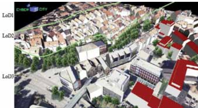
“Levels of Detail” (LoD) in CityGML, an application schema for Geography Markup Language 3 (GML3), the extendible international standard for spatial data exchange issued by the OGC and ISO TC211. Image courtesy of Dr. Steidler, CyberCity Modeler.
