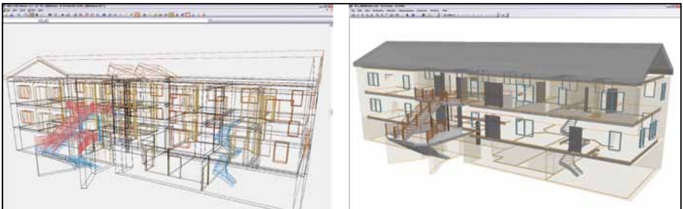
Figure 5. BIM IFC file shown as wireframe in IFC viewer and in ESRI's ArcScene application.
