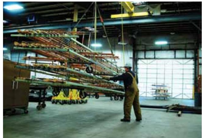
Figure 2. The set of 4 racks in the photo represents half a floor of laboratory piping and contains over 1,000 feet of pipe for 12 different systems.
