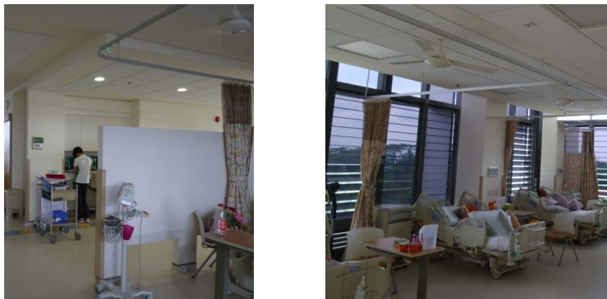
Figure A-4 Interior of naturally ventilated medical unit (Left: Partition wall; Right: Patient-controlled mechanical fans)
