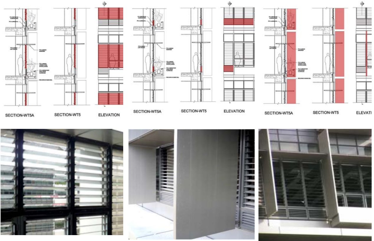
Figure A-3 Façade Design (Left: Jalousie Windows; Middle: Monsoon Windows; Right: Shading Devices/Wing Wall Design) (CPG Architects, 2009)
