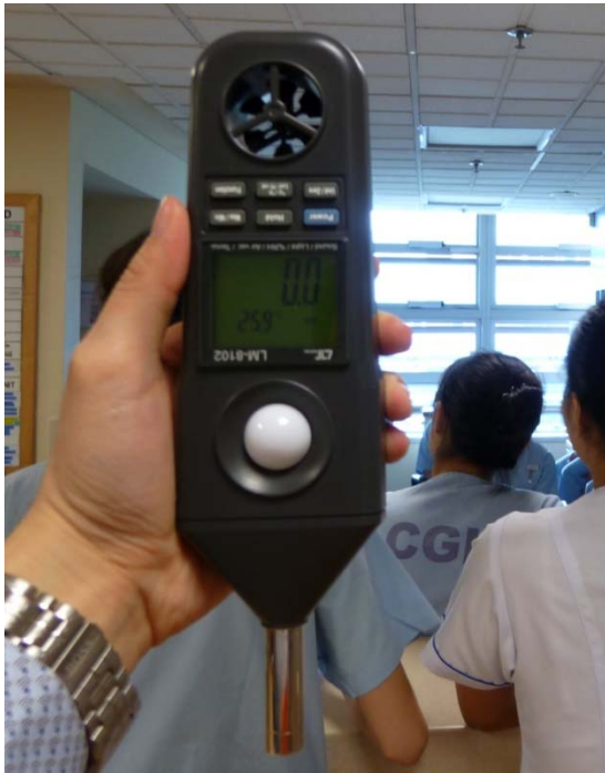
Figure 2-4 Thermal Environmental (TE) Meter
