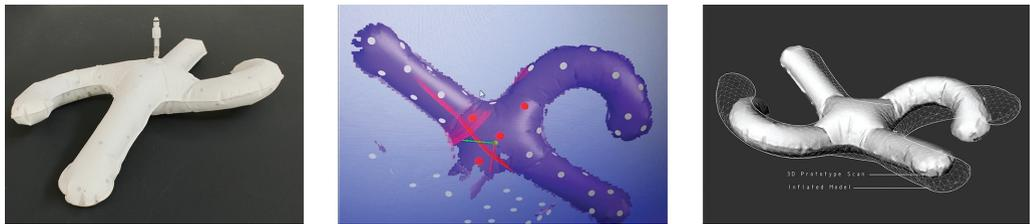
▲ Figure 9: l-r: X-Weave figure prototype, spray painted solid (for scanner detection) and tagged with laser scanning positioning dots; Screenshot of laser scanning data constructing a digital model; Overlay of digital model and scanned prototype figure. (Velikov/Thün 2014)
