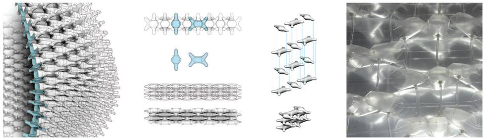
**X-Stack Prototype:** Aggregation through Stacking
