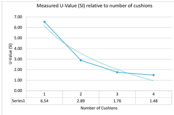
◀ Figure 14: Results of physical heat transfer test. Dashed is curve of control case and solid line illustrates measured thermal performance for one to four layers of 100mm deep cushions. (Velikov/Thün 2014)
