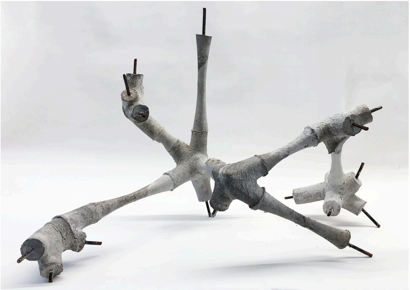
Resulting structural section cast in Rockite using PVA formwork and off the shelf #3 reinforcement. Bottom left - reinforcement is held in place by 3D printed jig. Bottom right: molds dissolve in a bath of water.
