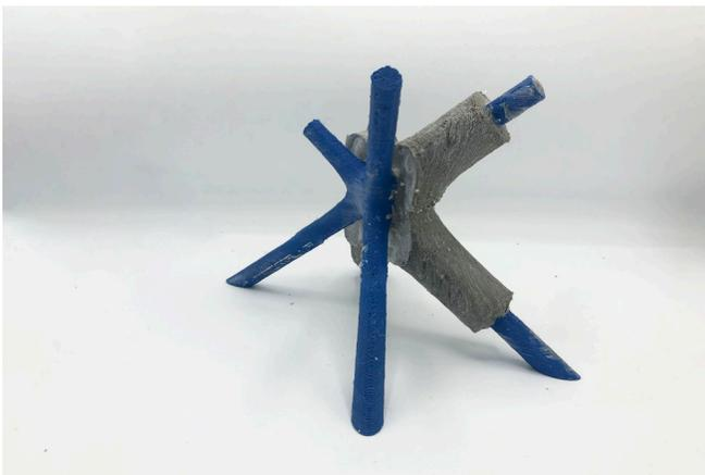
Images from top to bottom: Half completed PVA mold with #3 reinforcement, mold dissolving in water, complete cast with #3 reinforcement, half cast of Nylon X reinforcement
