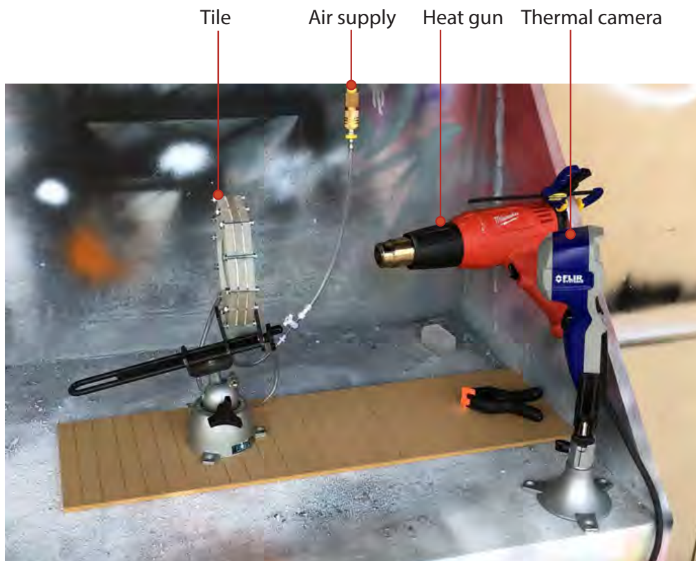
Figure 1. Image showing experimental setup. The tile is in the unheated position. The heat gun was held at varying distances so as not to overheat the tile. Temperature was recorded with the thermal camera. Printed or cast SMP tiles are fitted within the frame at left. Low pressure is supplied with a compressor and the SMP tile is heated to T_g with a heat gun.
