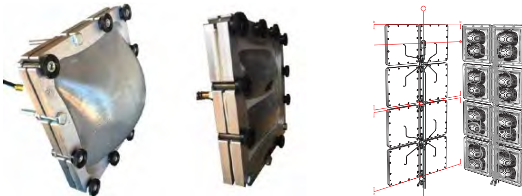
Figure 5: Test jig assembly 1 (for cast tiles) with composite hard plastic / shape memory polymer sample. The frame and silicone gaskets form a seal as air is held as constant pressure (1 psi). The tile is then heated to the T g temperature and the tile significantly deforms. The tile holds its deformed shape when the heat is removed. When reheated to T g the SMP tile returns to its original (casted or printed) shape.
