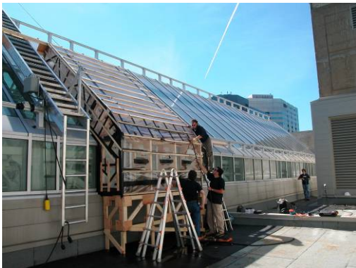
Figure 22: Exterior test chamber used to test a skylight section.
