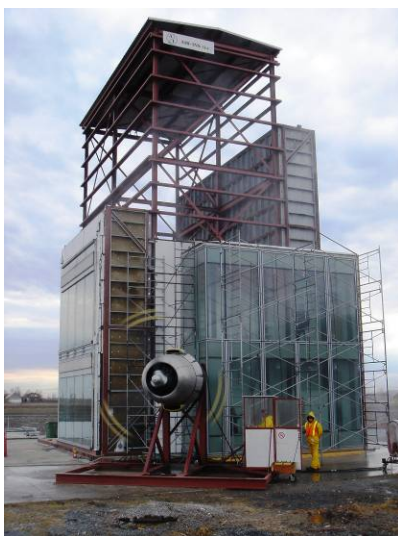
Figure 9: Exterior mock-up test (AAMA 501) - Air-Ins laboratory.
