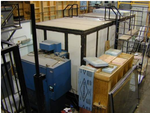
Figure 11: Environmental test chamber - Air-Ins laboratory.
