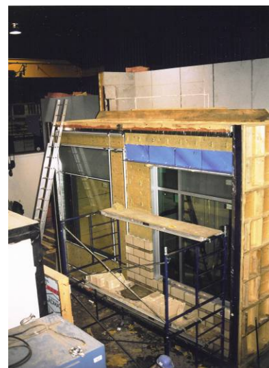
Figure 10: Interior mock-up test (CAN/CSA-A440) - Air-Ins laboratory.
