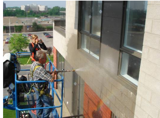
Figure 36: Diagnostic hose testing window/wall interface.
