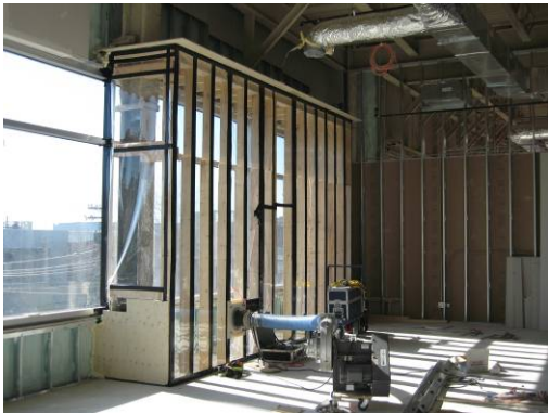
Figure 20: Interior test chamber used to test a portion of curtain wall section.
