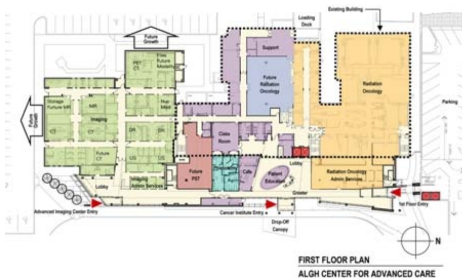
Image 3. First-floor plan for the new ALGH Center for Advanced Imaging Source: OWP/P
