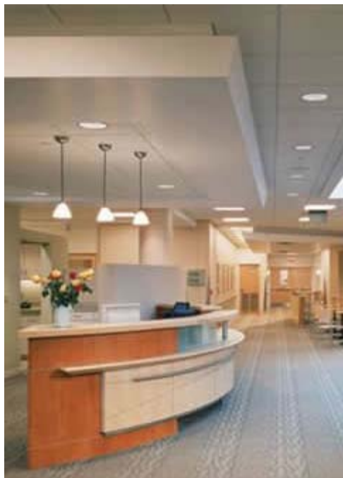
Pendant lighting at a nursing station helps to eliminate shadows on faces and functions as a wayfinding tool. 2
