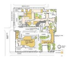
Replacement Plan Located on Same Site (Note improved site plan, demolition of old hospital and replacement facility)
