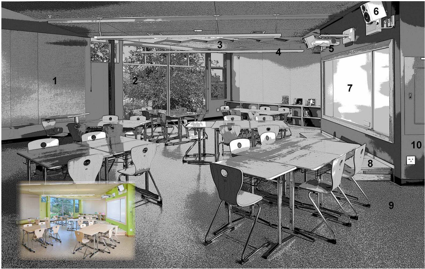
LEGEND 1. ACOUSTIC WALL TREATMENT 2. NORTH FACING GLAZING 3. ACOUSTIC CEILING TREATMENT 4. AUTOMATED LIGHTING SYSTEM 5. SHORT THROW PROJECTION SYSTEM 6. SOUND SYSTEM 7. LEARNING CENTER WITH STORAGE BEHIND 8. RETRACTABLE SPEAKING / PERFORMANCE PLATFORM 9. RUBBER FLOORING 10. LOW VOC PAINT Figure 7: Classroom Diagram Source: Trilogy Architecture
