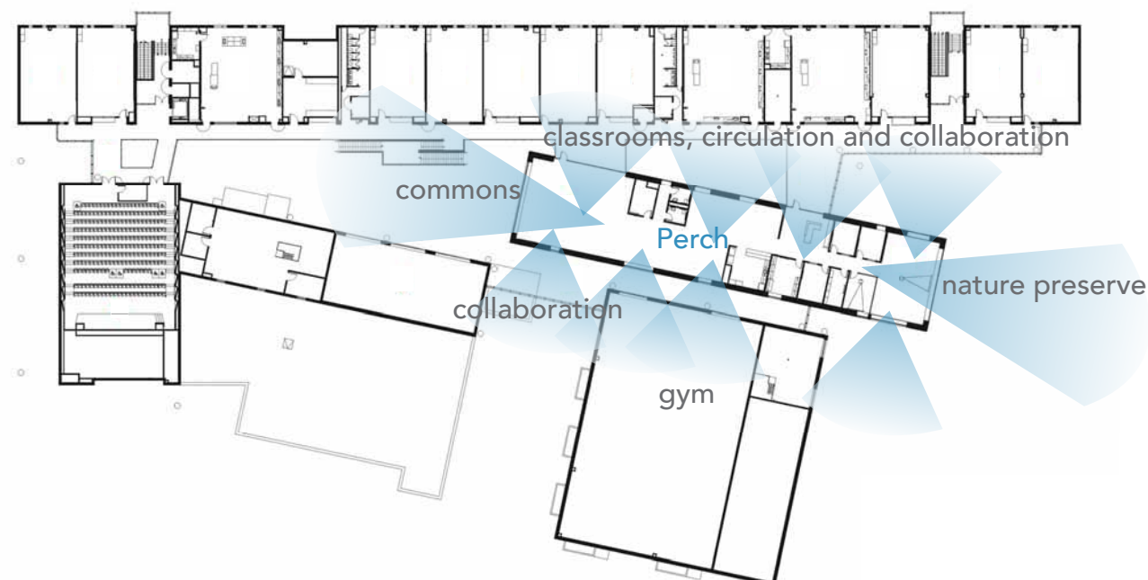
Figure 5: Perch Sight Lines Diagram: The diagram shows how the perch provides passive security throughout the building. Floor Plan Source: SHW Group
