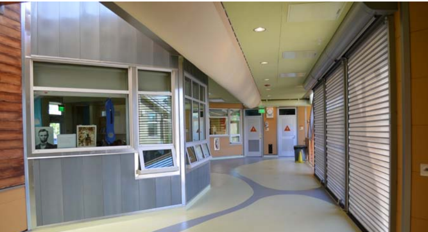
Image 35: Operable garage doors and the semi-conditioned space allow the classrooms to take advantage of natural ventilation.
