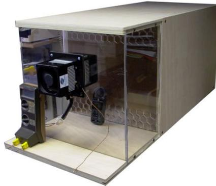
**Figure 4:** Desktop model with single A22 TE air cooler from Tellurex, inc installed in an double skin cavity of approx. 14”W x 14”H x 8”D. Insulation had not been applied to the enclosure when this image was taken.
