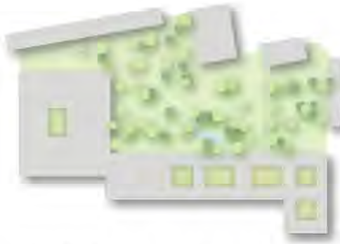
Figure 71: Perforated, articulated buildings with narrow building footprint to maximize daylighting and connections to nature, Hospital Basel, Switzerland.
