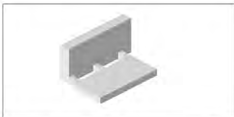
Figure 120: Unbundled hospital typology with patient tower and typically thick D&T block.
