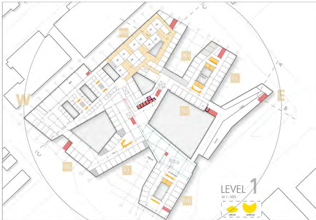
Figure 149: Floorplan level one illustrating the perforated building footprint of PACU and Surgery department (with facade matrix for shading concepts)
