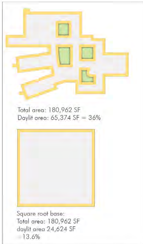
Figure 33: Daylight area of Dell Children's Hospital in comparison with its square root base.
