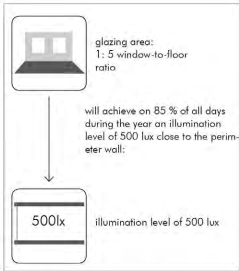
Figure 52: Size of glazing area and its relationship to interior illumination levels.
