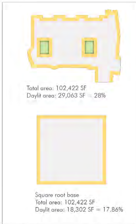
Figure 35: GGHC perimeter calculation for the diagnostic and treatment department of the Palomar Pomerado Health Medical Center, CA.
