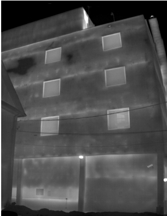
Figure 22. Negative Building Pressure (-140 Pa), T_o = 0^\circ\text{C} Figure 23. Positive Building Pressure (+40 Pa), T_o = 0^\circ\text{C} Both images taken during same evening, 4-hour time span between the two images.
