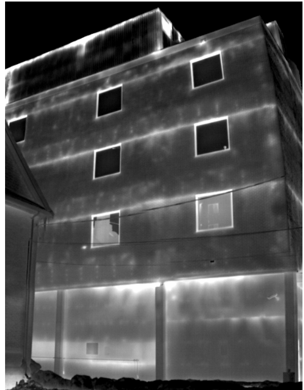
Figure 24. Negative Building Pressure (-8 Pa), T_o = -11^\circ\text{C} Figure 25. Positive Building Pressure (+25 Pa), T_o = -11^\circ\text{C}
