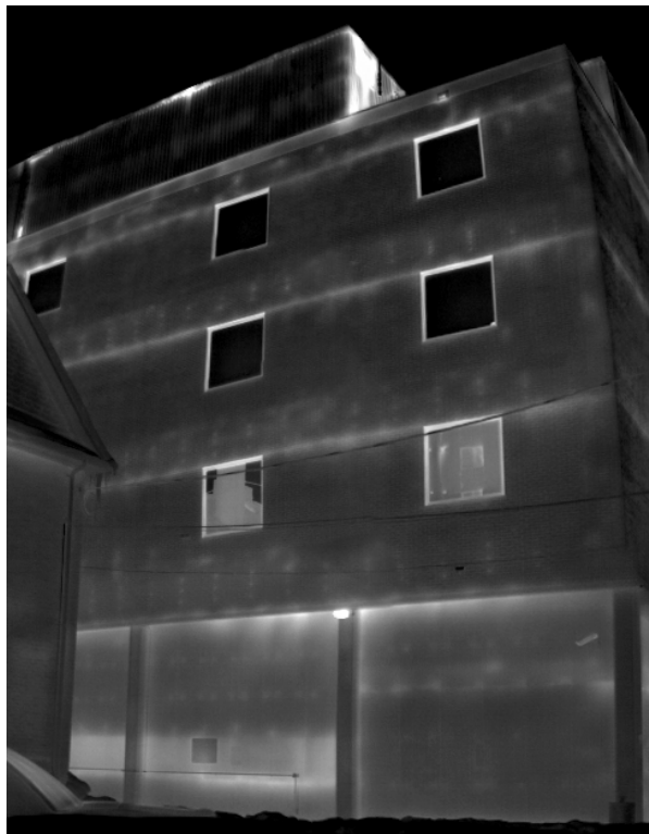
Figure 24. Negative Building Pressure (-8 Pa), T_o = -11^\circ\text{C} Figure 25. Positive Building Pressure (+25 Pa), T_o = -11^\circ\text{C}
