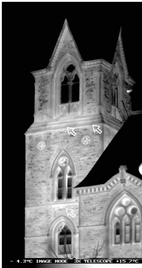
Figure 10. Neutral Building Pressure (0 Pa), T_o = -8^\circ\text{C} , No precipitation or snowfall for at least 7 days prior to inspection. Arrows point to suspected moisture accumulation within the limestone cladding due to rain and melt water throughout winter.
