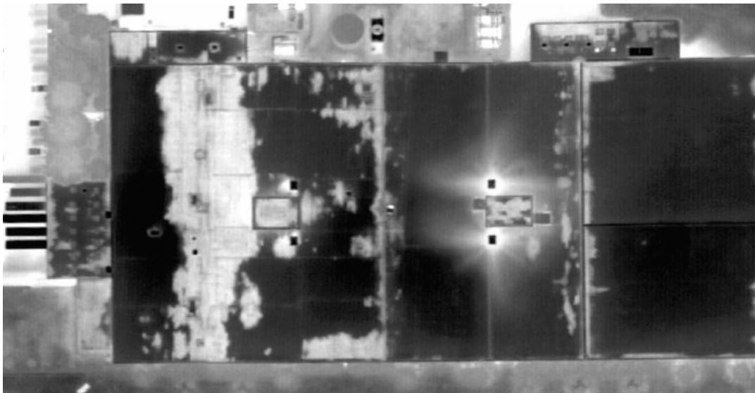
Figure 7; Aerial infrared image of moisture within insulation of conventional built-up roof. Note only one section of three requires replacement. The other two roof sections display minor roof leaks around curbs and flashings. (courtesy of AITScan and Stockton Infrared, Greg Stockton)
