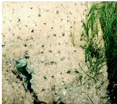
Figure 3: Biodegradable mat from the cellulose fibers that allow germinating seeds to sprout through the holes.
