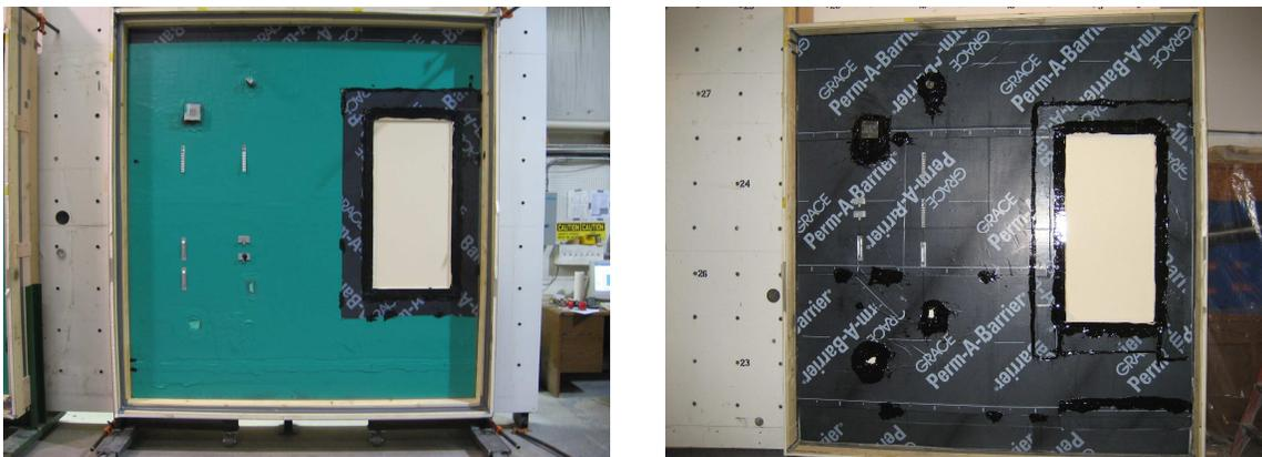
**Figure 9:** Full scale mock-ups of the installed air barrier assemblies complete with PVC pipe HVAC duct and electrical box penetrations sealed, windows flashed, tie-ins to roof and foundation and post-applied brick ties.
