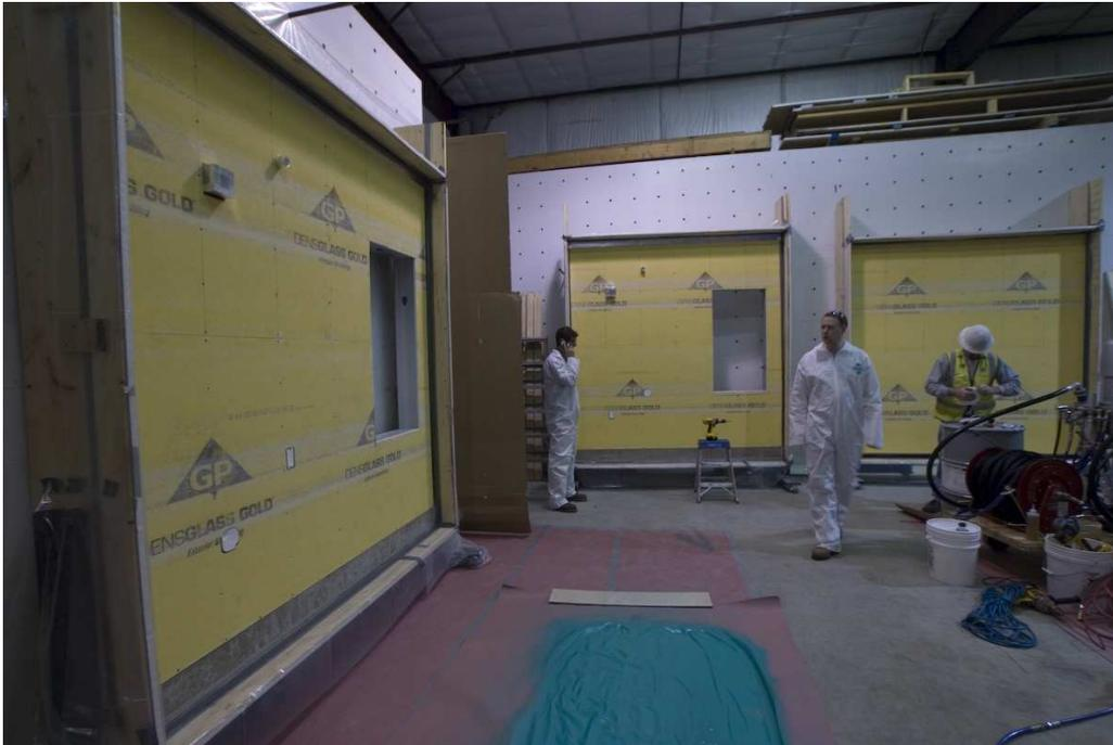
**Figure 5:** Photograph of wall specimens tested by Intertek. Each wall specimen was constructed according to ASTM E 2357 specifications.
