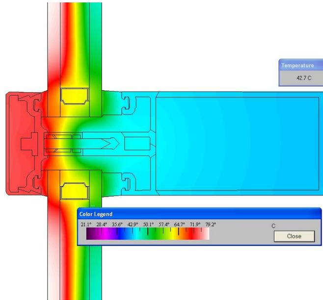
**Figure 5: Therm results for a dry glazed system with clear insulating glass and an aluminum IG spacer at an exterior temperature of 50C and 1120 W/m<sup>2</sup> solar load noting a 42.7 C frame temperature**
