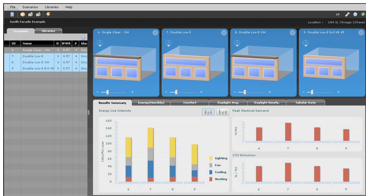
Figure 5. Scenario input screen of COMFEN comparing four design options.
