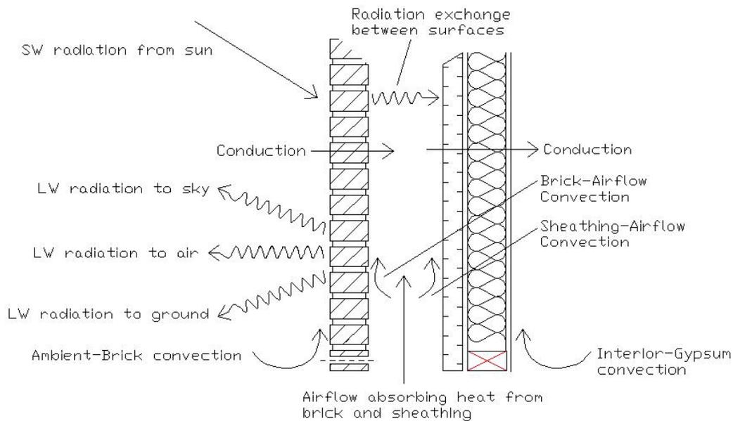
Figure 2 – Heat Transfer Mechanisms for a DBZ Wall
