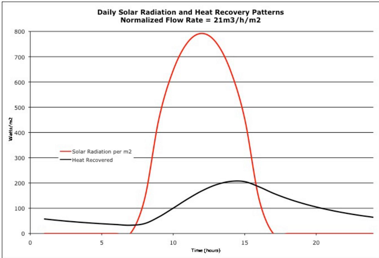
Figure 8 – Solar radiation per meter square and heat recovered daily patterns.
