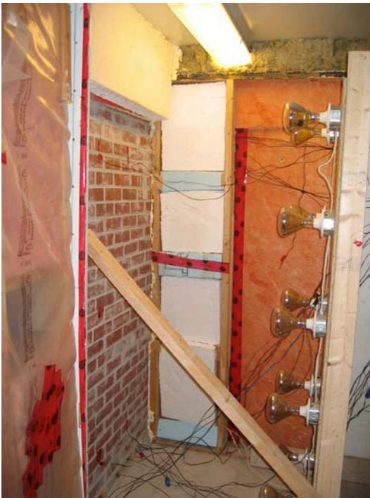
Figure 3 – Photograph of the Test Wall During Experimental Testing
