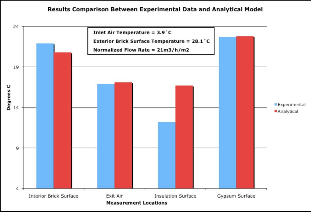
Figure 4 – Comparison of surface and air temperatures experiments and numerical model (21m<sup>3</sup>/h/m<sup>2</sup> normalized flow rate)
