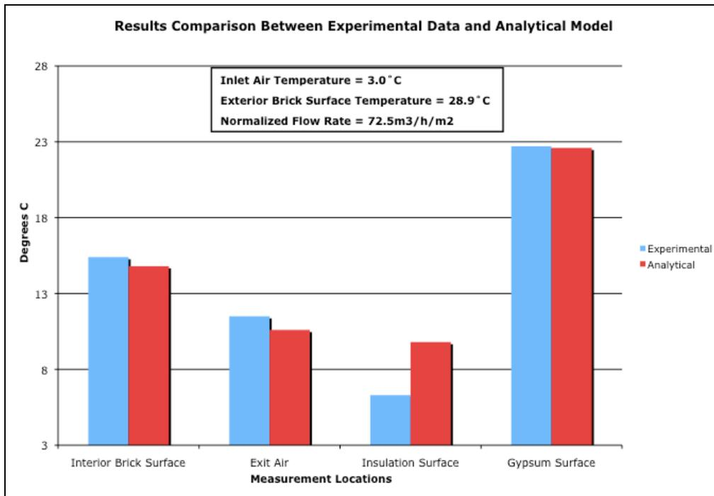
Figure 6 – Comparison of surface and air temperatures experiments and numerical model (72.5m<sup>3</sup>/h/m<sup>2</sup> normalized flow rate)
