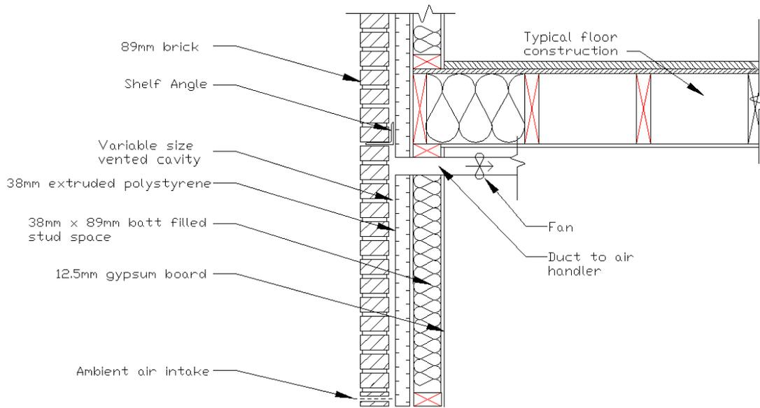
Figure 1 – Cross-sectional View of Conceptual Design
