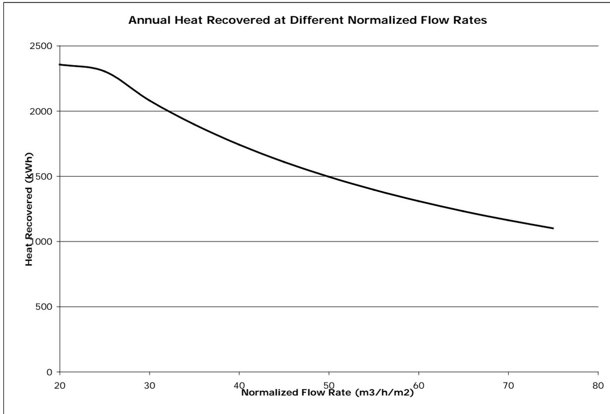
Figure 9 – Annual heat recovered at different normalized cavity flow rates.
