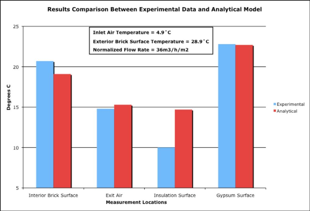
Figure 5 – Comparison of surface and air temperatures experiments and numerical model (36m<sup>3</sup>/h/m<sup>2</sup> normalized flow rate)
