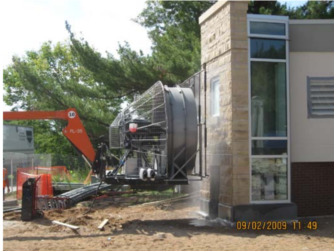
Figure 3: Dynamic water test being performed at an on site mock up
