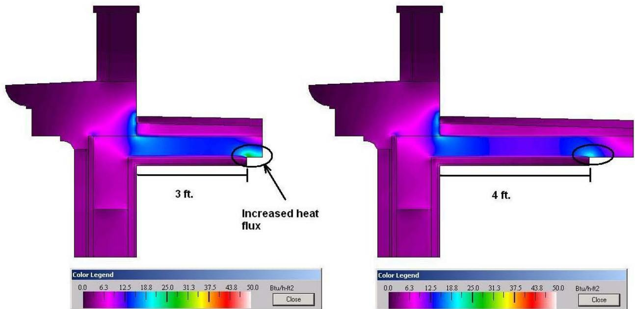
Figure 15. Temperature distribution at the roof parapet with for option with rigid insulation on the inboard surface of the CMU.
