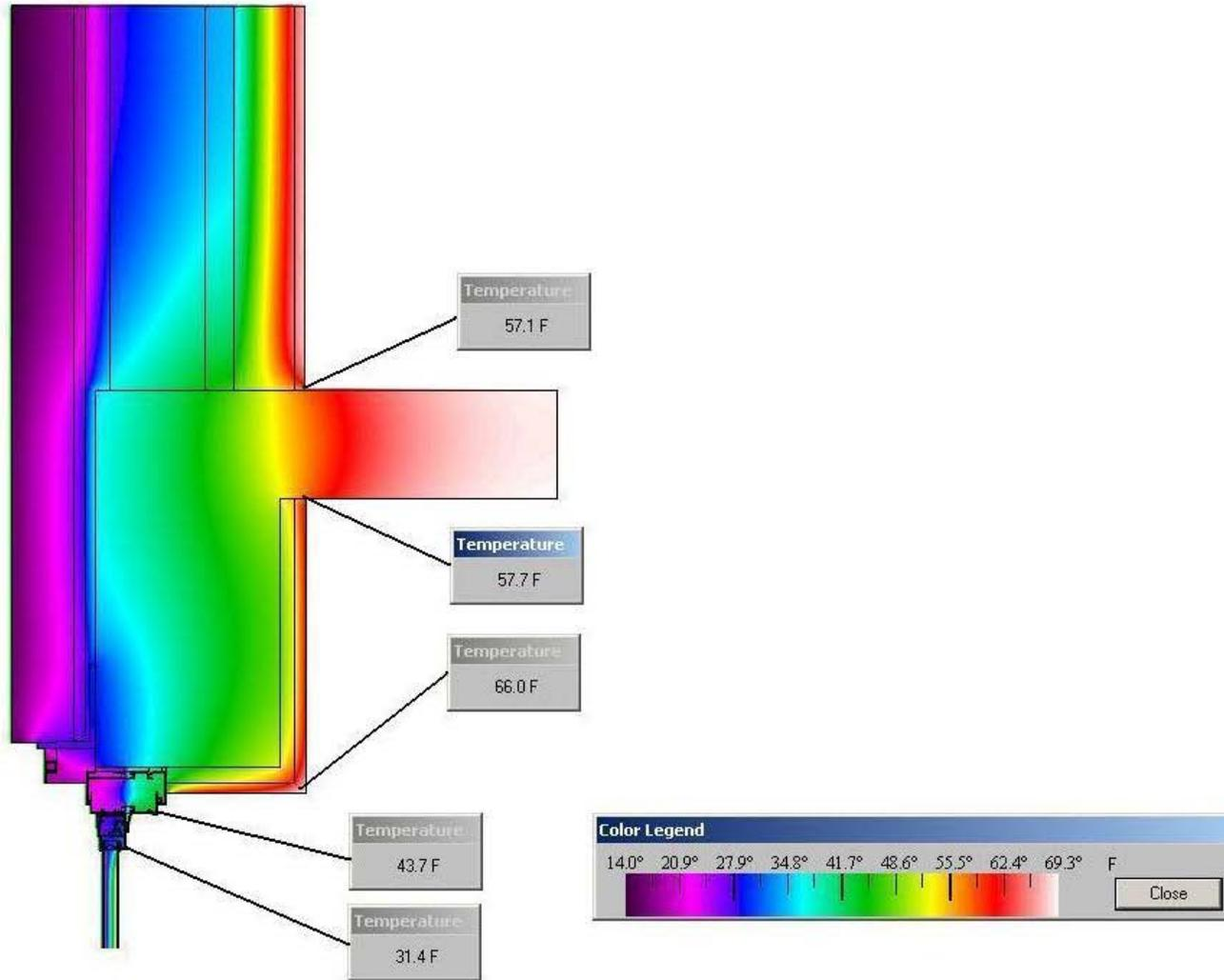
Figure 11. Temperature distribution through the wall assembly at the slab transition for remedial option with fiberglass insulation as proposed by the designer-of-record.
