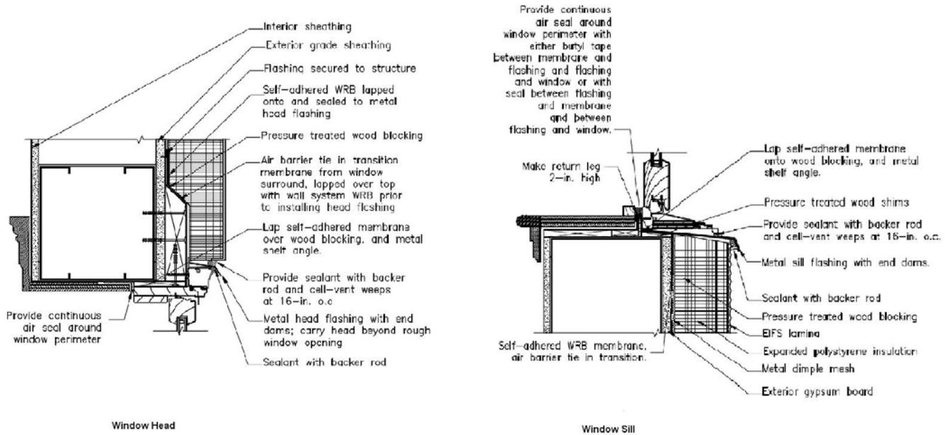
Figure 8. Air barrier transition at window sill and head.
