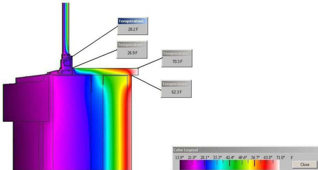
Figure 17. Temperature distribution at window-to-wall sill transition for option with fiberglass batt insulation.
