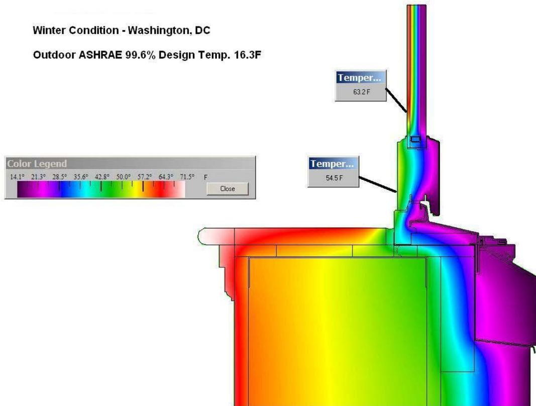
Figure 4. Temperature distribution at the window sill condition.
