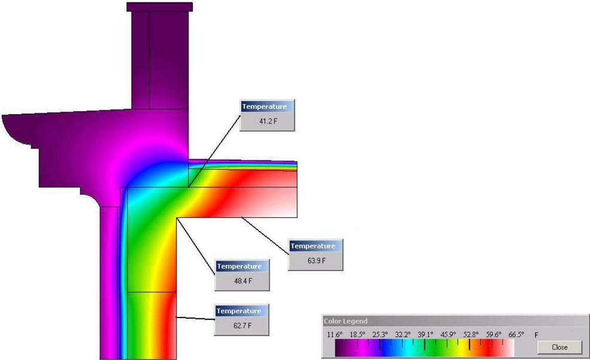
Figure 13. Temperature distribution at the roof parapet (existing condition).
