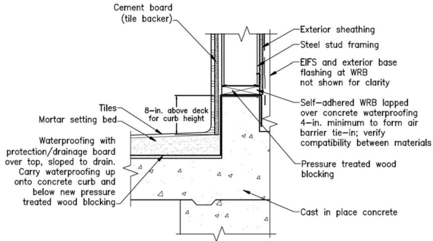
Figure 7. Air barrier transition at exterior pool wall-to-pool deck transition.
