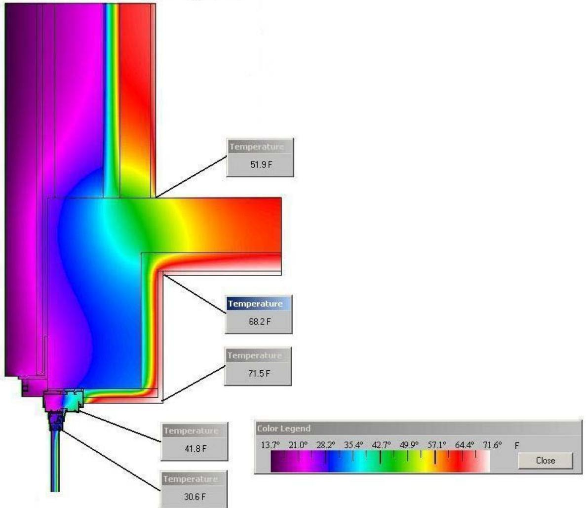
Figure 12. Temperature distribution through the wall assembly at the slab transition for alternative option with rigid insulation on the inboard surface of the CMU.
