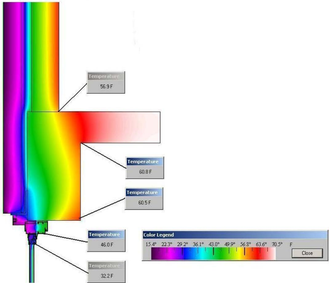
Figure 10. Temperature distribution through the wall assembly at the slab transition (existing condition).
