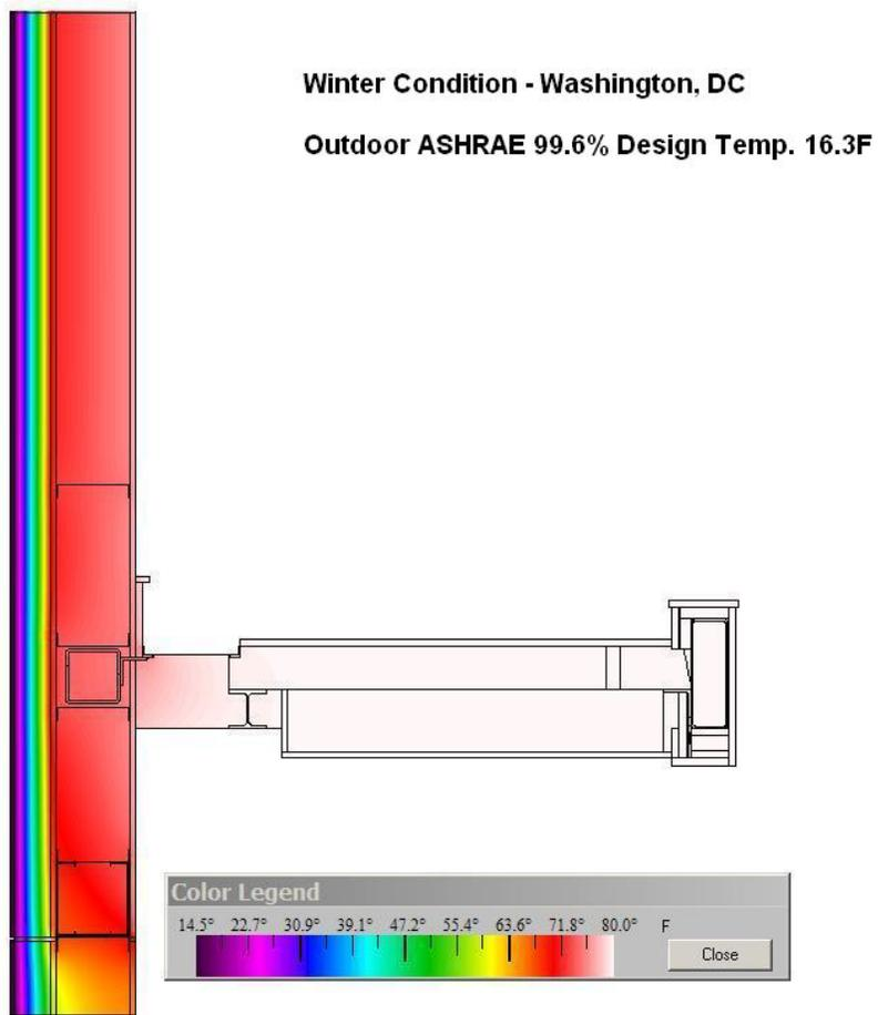
Figure 2. Temperature distribution through proposed and thermally improved wall-to-window transition at sill.
