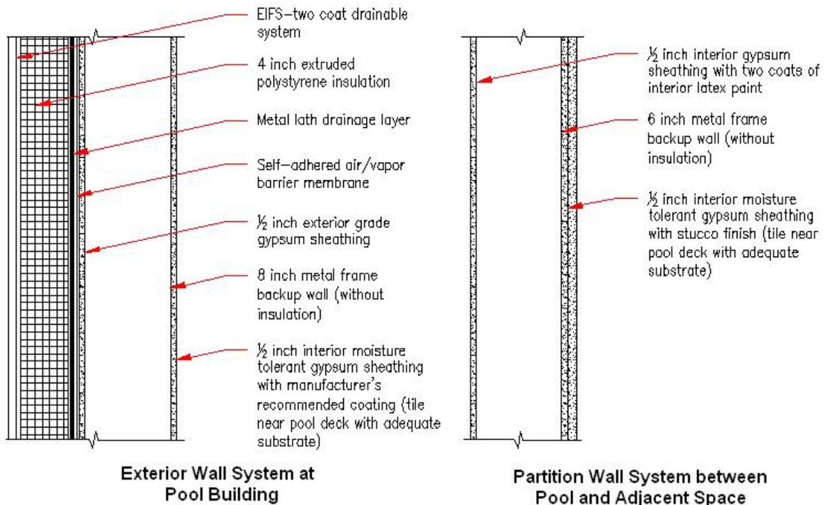
Figure 1. Proposed wall system for the new pool building addition.
