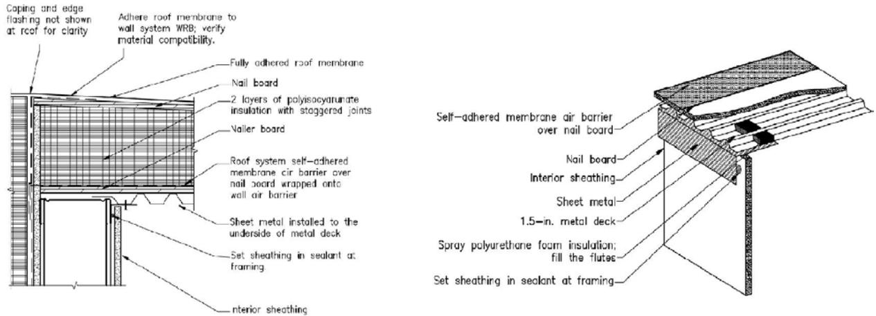
Figure 6. Air barrier transition at exterior pool wall-to-roof deck transition.
