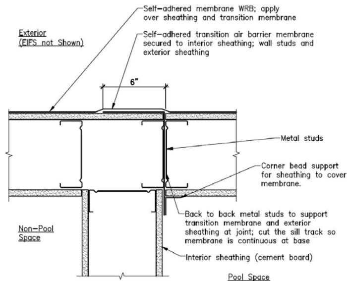
Figure 5. Air barrier transition at exterior pool wall-to-partition wall transition.
