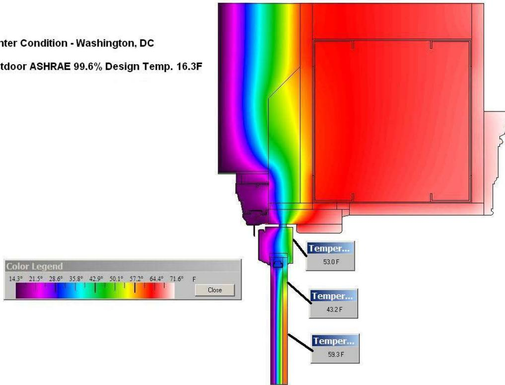
Figure 3. Temperature distribution at the window head condition.
