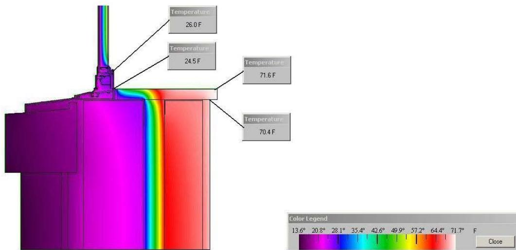
Figure 18. Temperature distribution at window-to-wall head transition for option with rigid insulation on the inboard surface of the CMU.
