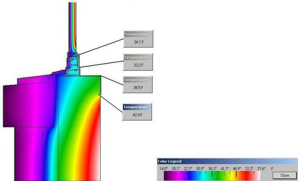
Figure 16. Temperature distribution at window-to-wall sill transition (existing condition).
