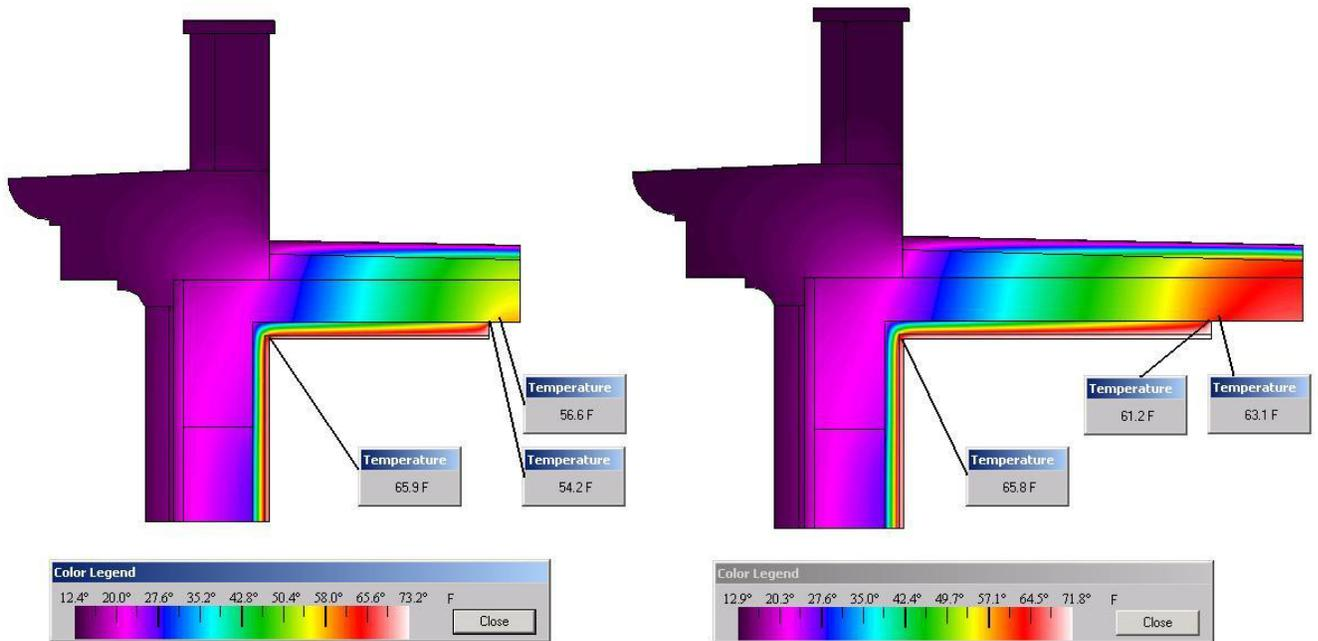
Figure 14. Temperature distribution at the roof parapet with for option with rigid insulation on the inboard surface of the CMU.
