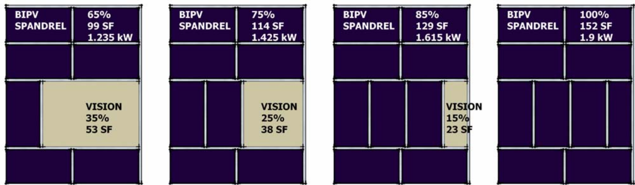
Fig. 3: Variations in percentage of BIPV spandrel and vision glazing.
