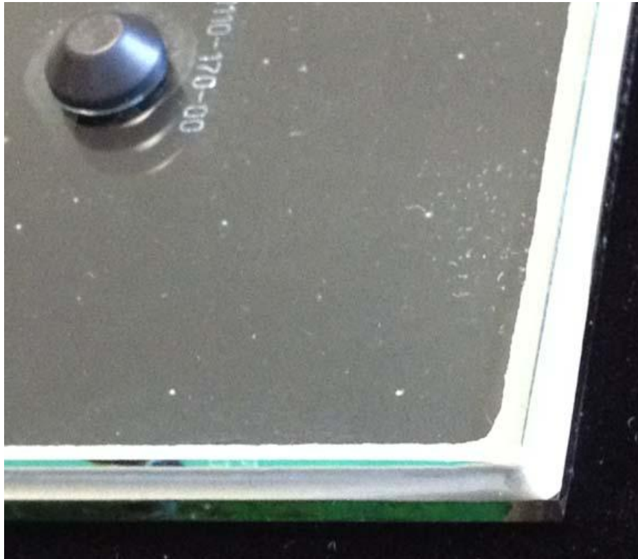
Fig. 13 Corner detail of rigid solder glass seal
