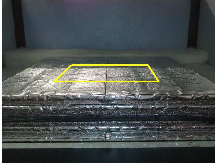
FIGURE 4: Situation B1, single joint in one layer with vertical projected measuring zone (yellow) of the guarded hot plate
