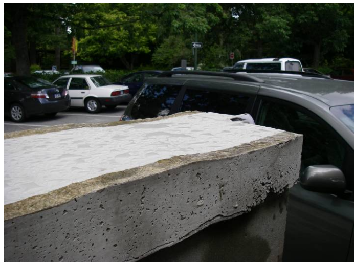
FIGURE 8: PMMA Membrane Test on Puddled Earth Cap
