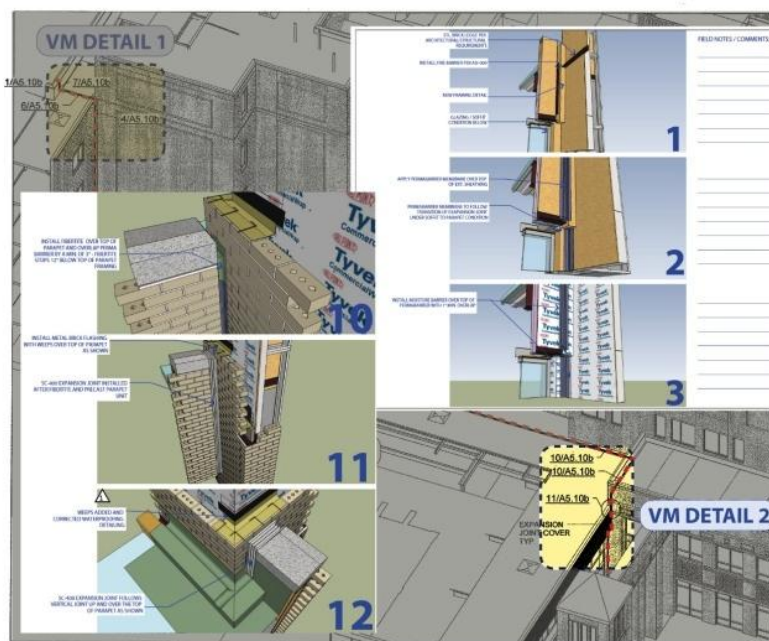
Figure 6. Mortensen Construction (Contractor) used Google Sketchup to model select building envelope corner section for coordination between design and construction teams.
