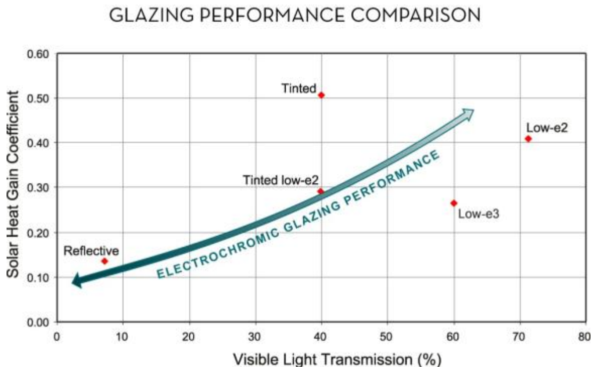
Figure 1: Graph of visible light transmission ( T_{vis} ) versus solar heat gain coefficient (SHGC): This chart shows the heat gain and light transmission range of a high performance EC product compared with some examples of standard static glass.
