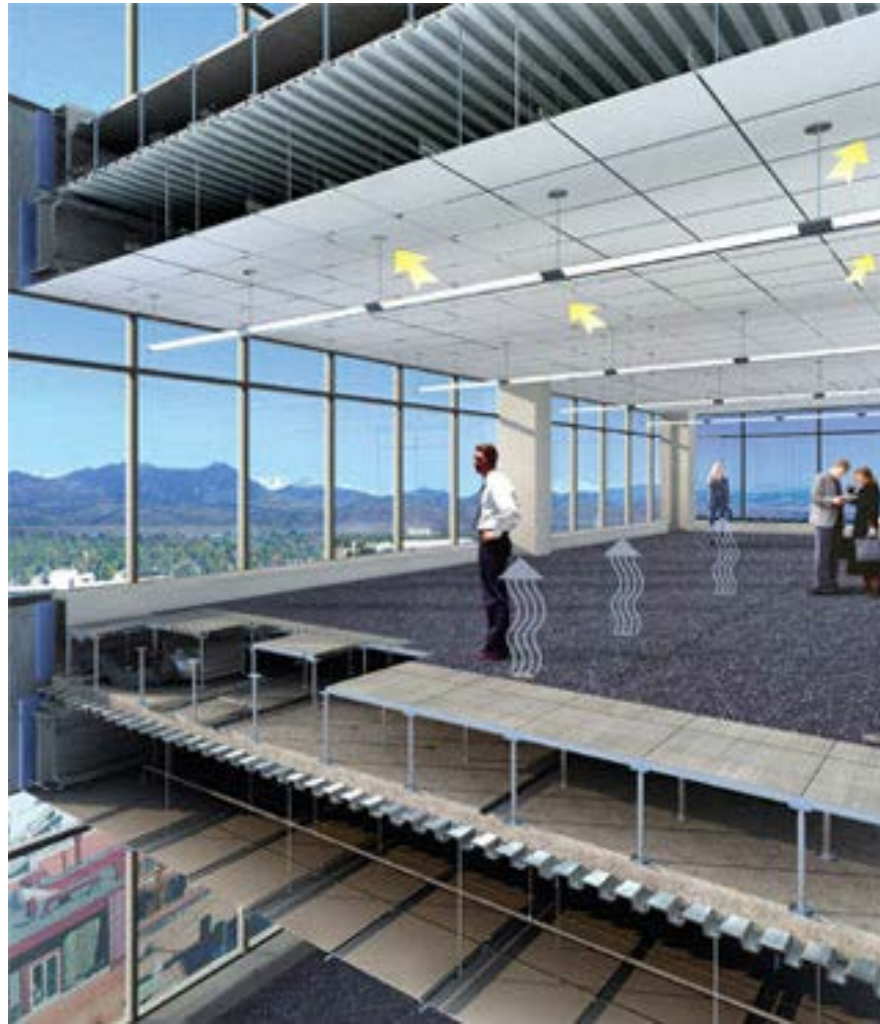
Figure 8 - UFAD with Perimeter Fan Powered VAV Boxes
