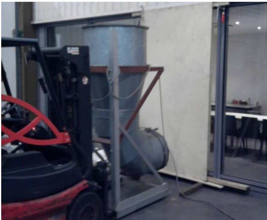
Figure 4. Dynamic testing with axial fan and mounted spray nozzle (ENV 13050:2000)
