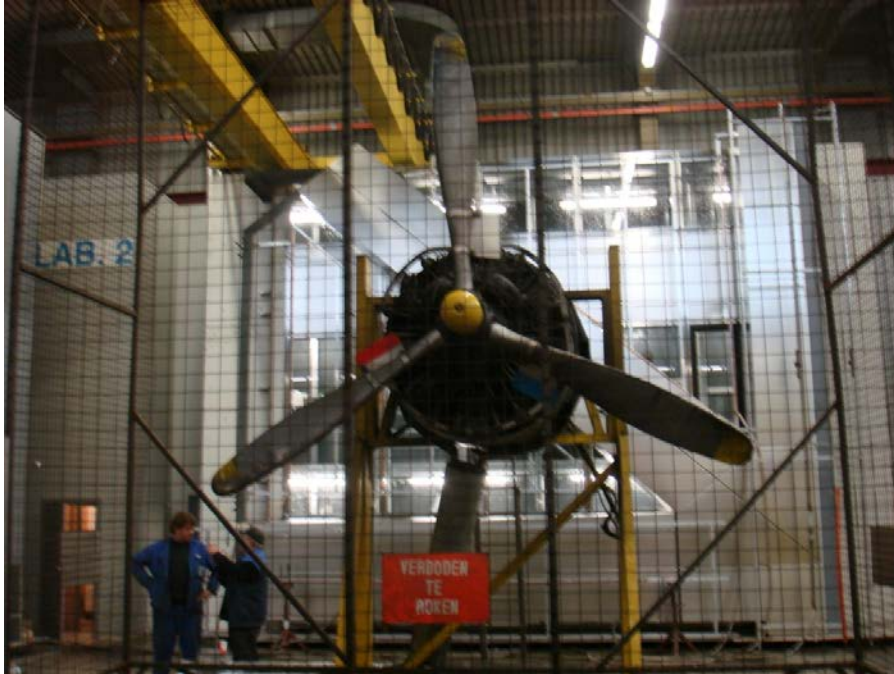
Figure 3. Dynamic test with aero-engine (AAMA 501.1:2004)
