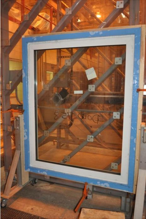
Figure 9. Air Testing set-up of Dow Corning® 758 Silicone Weatherbarrier Sealant
