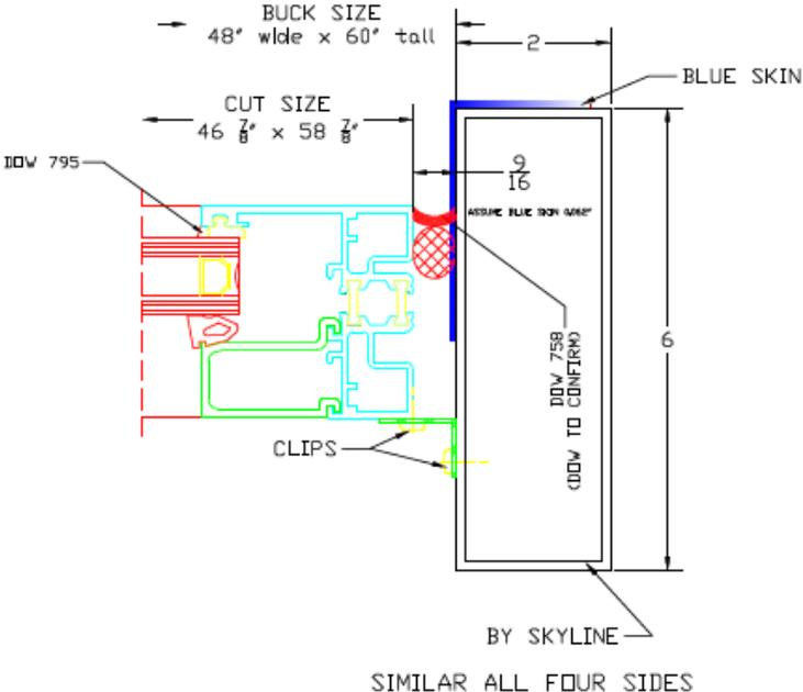
Figure 8. Sample Test Detail
