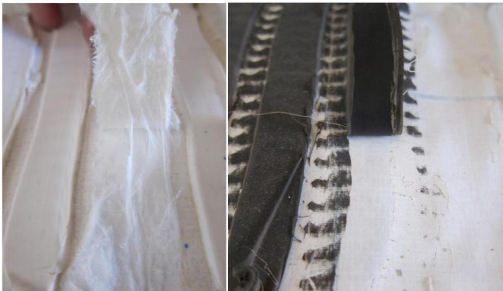
Figure 6: Adhesion of polymer/resin blend sealant (left) and a common silicone sealant (right) after 2 years in Phoenix Desert Outdoor Weathering Site, to a common spun bound polyolefin weather barrier membrane
