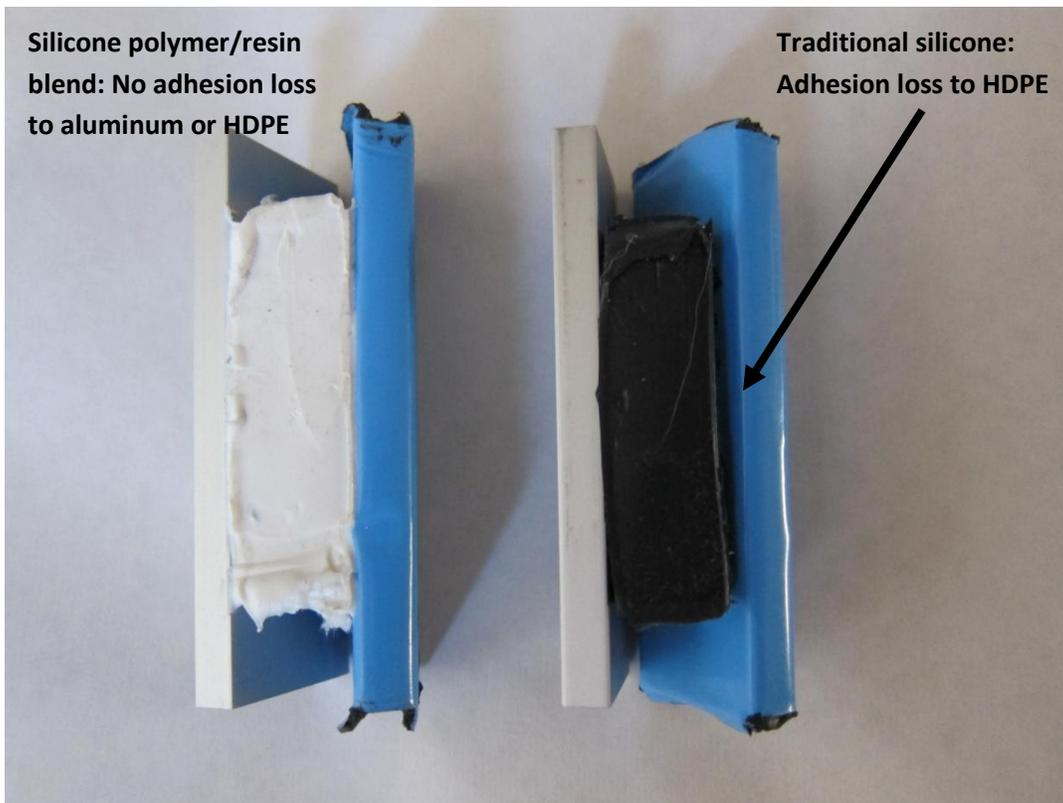
Figure 7: Polymer/resin blend sealant joint after being tested for +/- 25% movement (left) and standard silicone sealant joint after being tested for +/- 25% movement (right). Substrates are anodized aluminum and HDPE.
