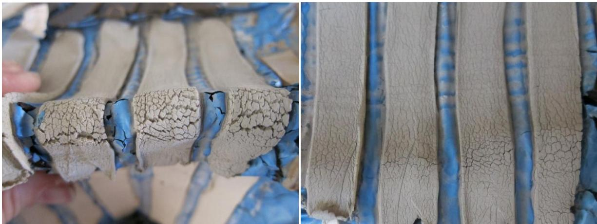
Figure 4: Organic technology sealant after 2 years in Phoenix Desert Outdoor Weathering Site. No cleaning or special preparation of the sealant. Substrate is a common SAF weather barrier membrane.
