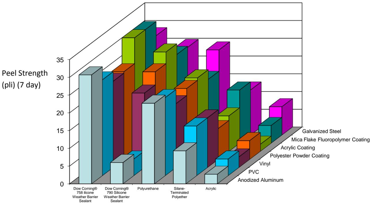
Figure 1: Adhesion of sealants to common building substrates.
