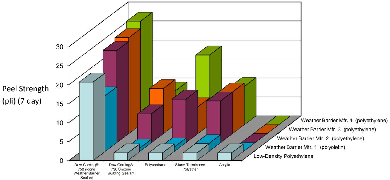
Figure 2: Adhesion of sealants to weather barrier substrates.
