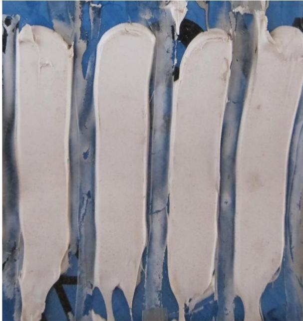
Figure 3: Silicone Polymer Resin Blend Sealant after 2 years in Phoenix Desert Outdoor Weathering Site. No cleaning or special preparation of the sealant. Substrate is a common SAF weather barrier membrane.
