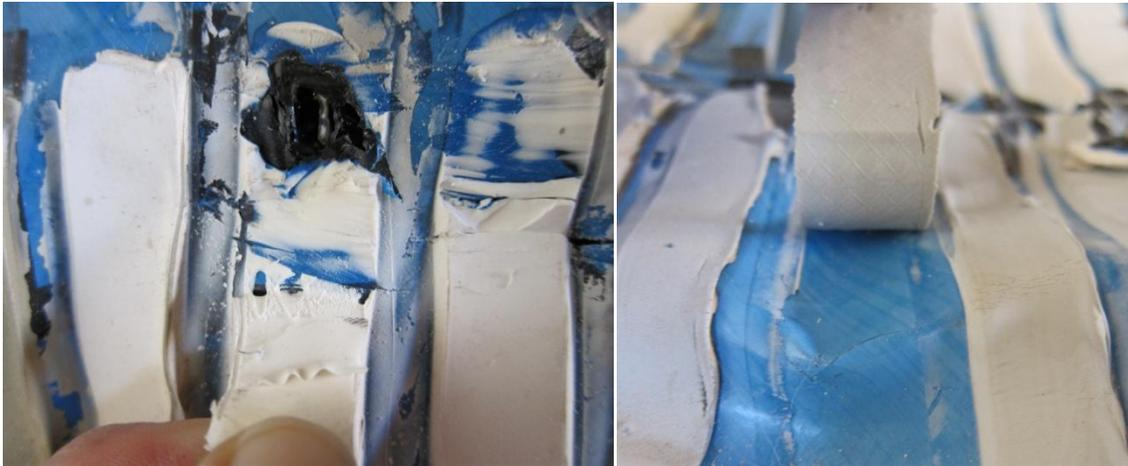
Figure 5: Adhesion of polymer/resin blend sealant (left) and a common silicone sealant (right) after 2 years in Phoenix Desert Outdoor Weathering Site, to a common peel and stick weather barrier membrane with a high density polyethylene top sheet.
