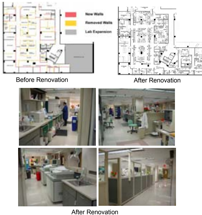
Figure 31. Renovation from Compartmentalized Lab to Semi-Open and Flexible Lab, St. Clare's Hospital
