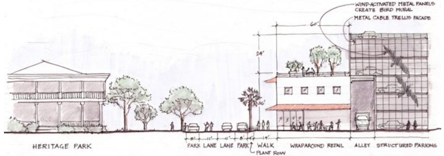
In this section a future parking structure is fronted by pedestrian oriented retail along Chaparral and a new parking garage for the convention center is wrapped with a wind activated mural, celebrating the city's unique avian assets.
