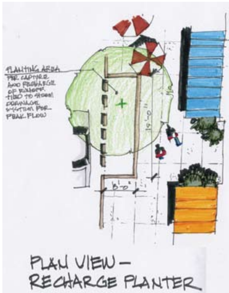
Above: Plan view of recharge planters. An example of regenerative green infrastructure – the new sidewalk planters act as storm water treatment for surface water.
