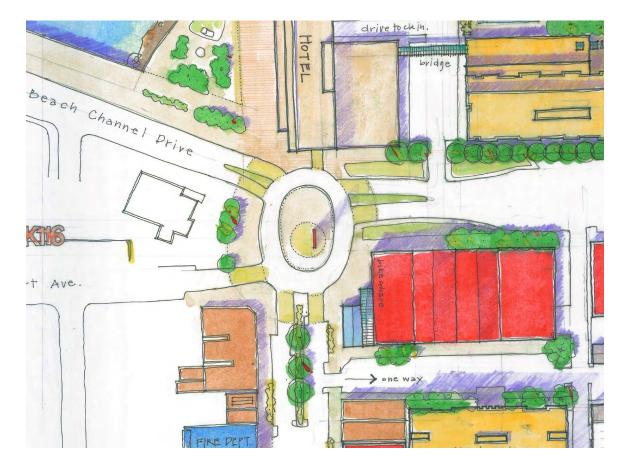
A single oval shaped roundabout can be designed to accommodate all of the traffic at this site. Consolidating two intersections into one simplifies the intersection and dramatically reduces the risk and severity of collisions.
