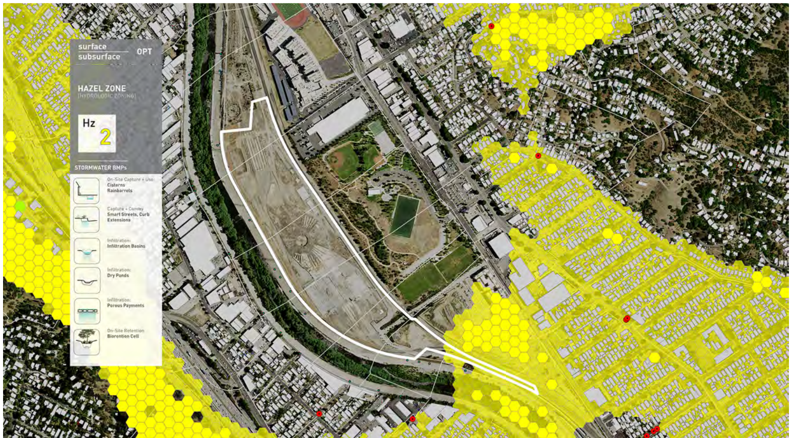
Figure 8: Locations of stormwater management opportunities within Hazel Zone 2 at neighborhood scale. Hazel provides BMP prioritization: darker yellow hexagonal markers indicate areas of higher priority (less expensive capital costs due to improved surface and subsurface conditions as compared with areas of lighter yellow markers.).
