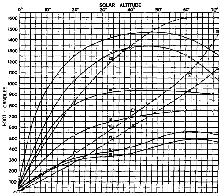
Fig. 5.—Curves of summer skylight illumination intensity on different surfaces. Curve I. Clear sky. Vertical surface facing 0^\circ in azimuth from sun. Curve II. Clear sky. Vertical surface facing 45^\circ in azimuth from sun. Curve III. Clear sky. Vertical surface facing 70^\circ in azimuth from sun. Curve IV. Clear sky. Vertical surface facing 90^\circ in azimuth from sun. Curve V. Clear sky. Vertical surface facing 135^\circ in azimuth from sun. Curve VI. Clear sky. Vertical surface facing 180^\circ in azimuth from sun. Curve VII. Clear sky. Horizontal surface. Curve VIII. Cloudy sky. Horizontal surface. (Note: Double the intensity scale). Curve IX. Cloudy sky. Vertical surface.
