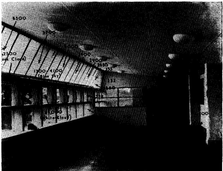
Figure 12. Luminance measurements are transferred to Petherbridge's diagram, and the combined source luminance, source size, and position factors determined together.
