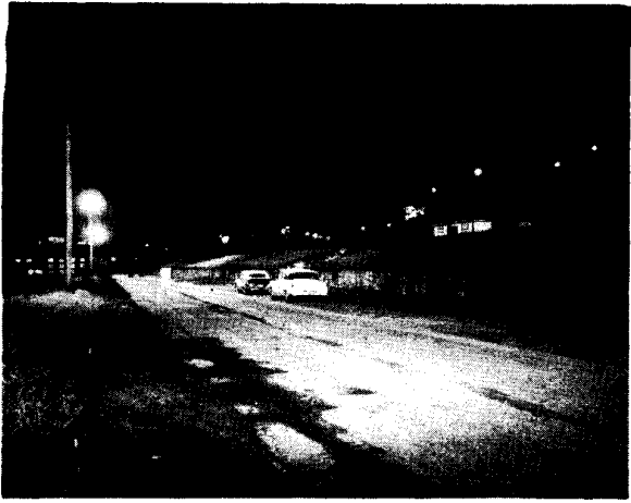
Figure 6. Test installation with general purpose floodlights and open suburban units turned on.
