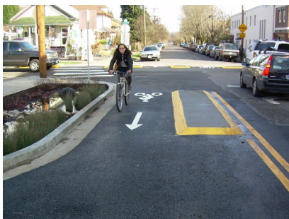
Streets are converted to bike boulevards with signage, striping and minimal medians.
